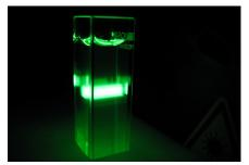
In spectroscopy, fluorescence is one of the more challenging setups, due to low fluorescent emission (about 3% of the excitation energy). The AvaSpec-ULS2048CL-EVO gives the highest sensitivity and the AvaLight-LED series provides excitation at the requested wavelength.
